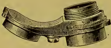
Fig. 163.—Watson's Centring Nose-piece of Microscope.
